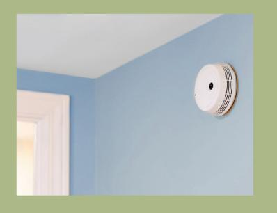
Smoke detectors should be installed in every bedroom, out side of every sleeping area and on every level including basements.
